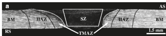
Figure 2. A typical macroimage of different microstructural zones in a FSWed material (reproduced from [94], with permission from Springer, 2017).
