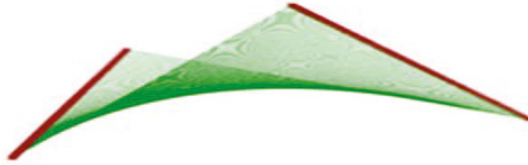
Figure 3. A hyperbolic paraboloid with the directrix lines expressed.
