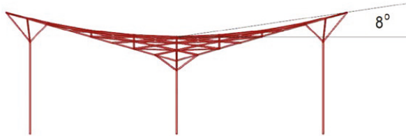
Figure 6. Determination of the roof inclination angle.
