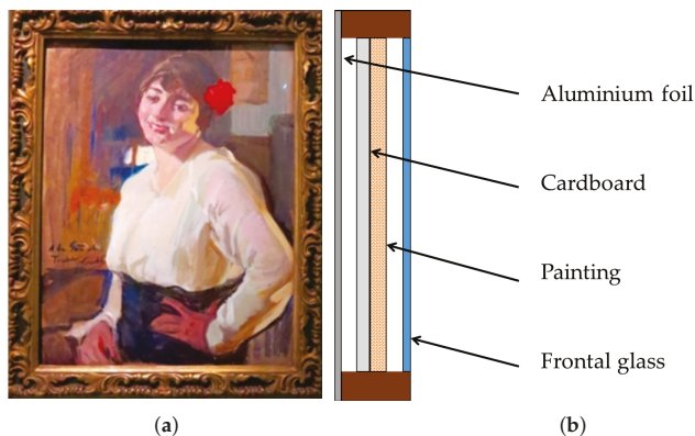
Figure 1. Portrait on cardboard titled “Portrait of a lady with a red flower in her hair” by J. Sorolla (a); and schematic cross section of the microclimate frame used and layout of its components (b).
