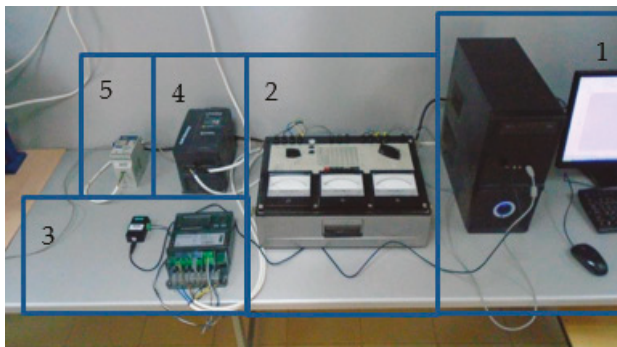
Figure 6. A set of measuring equipment used for the research. 1—personal computer; 2—K-505; 3—Mercury 221 electric energy meter with USB-CAN/RS-232/RS485 adapter; 4—frequency converter Hyundai N700-220HF; 5—circuit breaker
