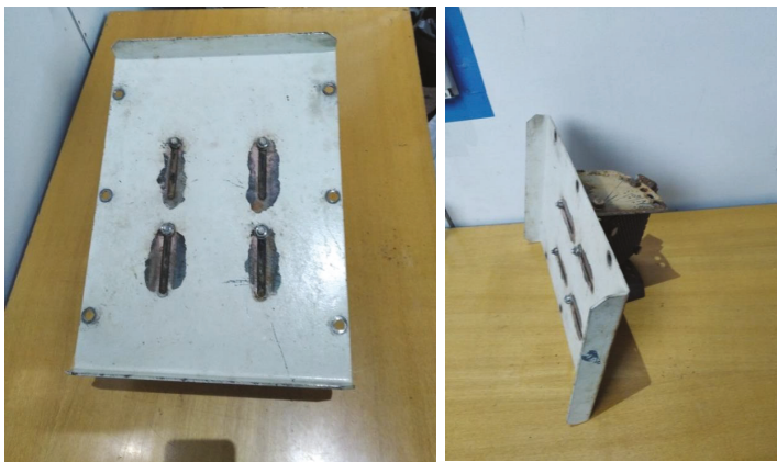
Figure 6. Cover with slots for adjusting the clearance S between the grid-work (plate) and the nozzle.
