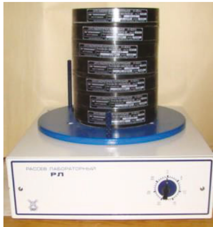
Figure 11. Laboratory plensifter RL brand with a set of sieves for determining the granulometric composition of the forage.
