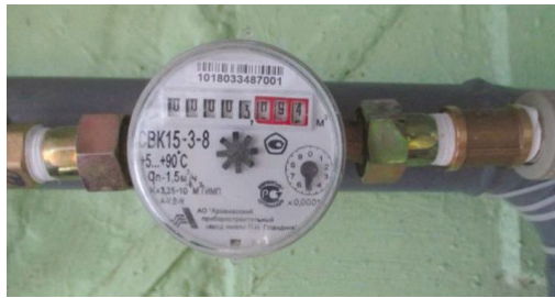
Figure 2. Water meter SVK 15-3-8 used for recording the amount of water poured into the tank of the measuring station.
