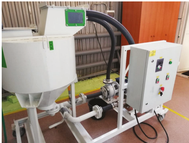
Figure 1. The measuring station for preparing forage from grain.
