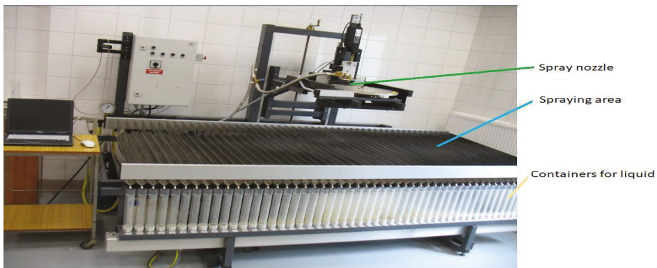
Figure 1. Measurement table (Department of Machinery Exploitation and Management of Production Processes, University of Life Sciences in Lublin).
