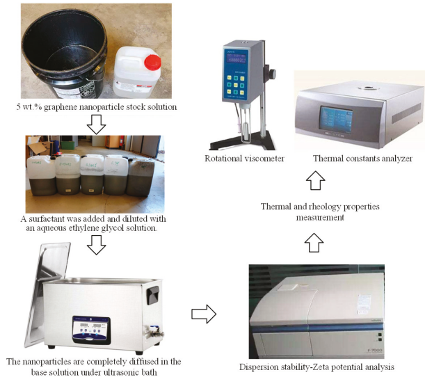
Figure 3. Graphene nanofluid preparation and the physical property measurement process.
