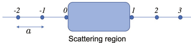
Figure 1. Schematics of the model of a scattering (shaded) region connected with two semi-infinite one-dimensional leads.
