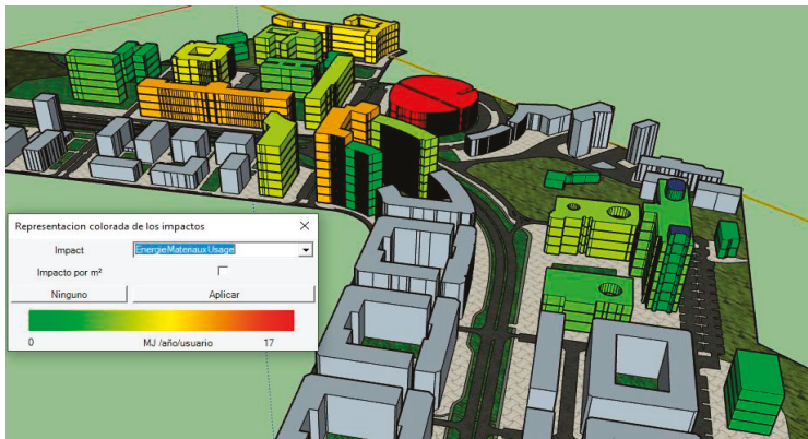
Figure 6. Graphical evaluation of the simulation of impacts for the campus with NEST.
