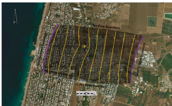
Figure 4. 2D numerical model domain and boundary conditions of the Nahariya site: yellow lines represent the simulated groundwater heads.
