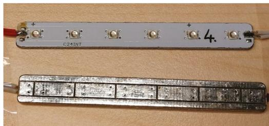
**Figure 13.** The sample mid-power LEDs mounted on FR4 strips; the printed circuit boards were provided with increased thermal interfaces for better cooling capabilities.
