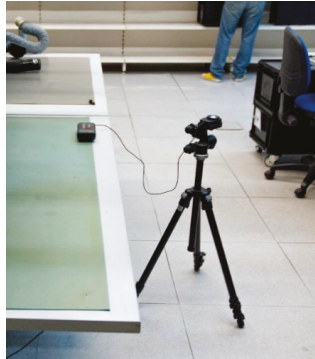
Figure 7. Illuminance measurement procedure in a lighting survey. A T-10a Minolta calibrated illuminance meter was used for the measurements.
