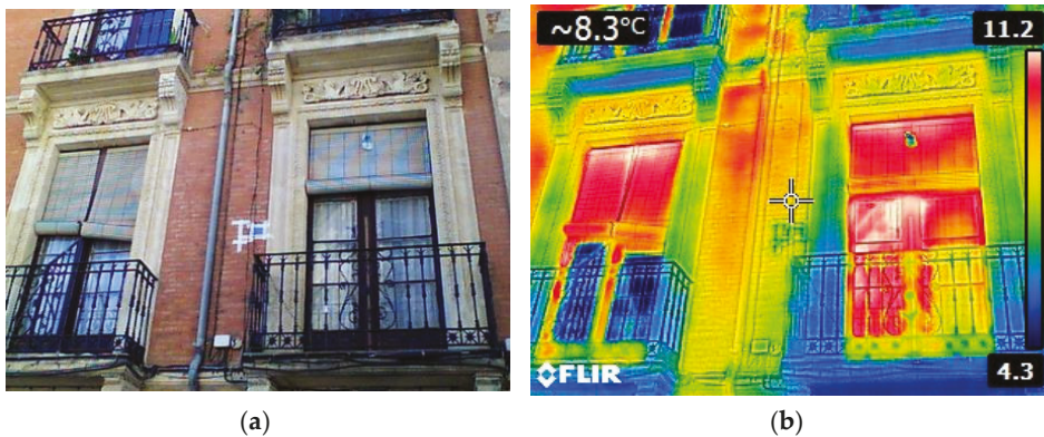
Figure 1. (a) Placement of the thermal flow plate and probes on the exterior face of the facade; (b) Thermographic image of the facade.
