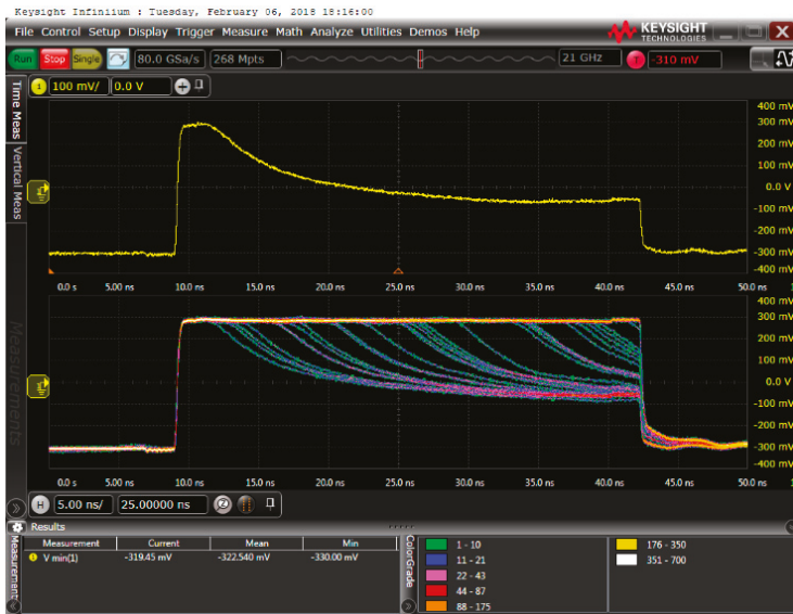
Figure 5. Oscilloscope picture of one avalanche ( top ) and several overlaid avalanches ( bottom ) of the cathode voltage of a SPAD type B with 48.2 \mu\text{m} diameter for an illumination power with a halogen source to achieve somewhat equally distributed photon hits.
