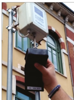
Figure 10. Operation of calibration on DYNAMAP sensor.
