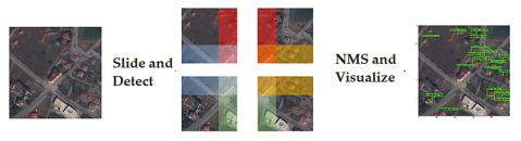
**Figure 6.** Process of the proposed detection flow of a  $500 \times 500$  image with 100 pixels overlapping; the colored parts in the middle represents overlapping areas.
