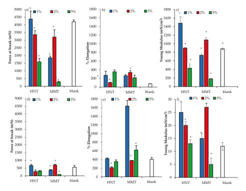
**Figure 8.** Mechanical properties (force at break mN, **a**–**c**; elongation %, **b**–**e**; Young's Modulus mN/cm<sup>2</sup>, **c**–**f**) for dry (**a**–**c**) and wet (**d**–**f**) scaffolds loaded with HNT or MMT at different concentrations (mean values  $\pm$  SD; n = 3). Statistics: \* = Mann–Whitney (Wilcoxon) W test *p* < 0.05.
