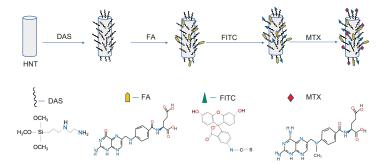
**Figure 2.** Schematic representation of the conjugation of both FA and FITC to DAS which is attached to the HNT surface. Methotrexate (MTX) was vacuum-doped into the HNT lumen. DAS = N-[3-(trimethoxysilyl)propyl) ethylenediamine, FA = folic acidity, FITC = fluorescein isothiocyanate.
