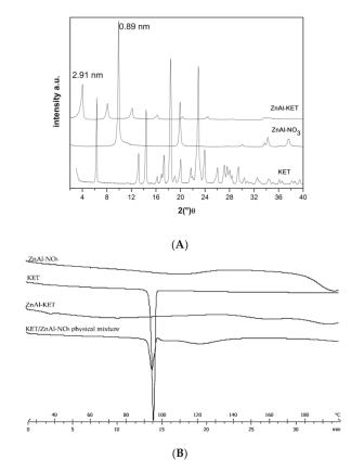
**Figure 1.** (**A**) XRPD pattern (X-ray diffraction patterns) of crystalline ketoprofen (KET) (acid form), pristine ZnAl-NO<sub>3</sub>, and the hybrid ZnAl-KET. (**B**) Thermal profiles measured by differential scanning calorimetry of ZnAl-NO<sub>3</sub>, crystalline KET, ZnAl-KET, and KET/ZnAl-NO<sub>3</sub> physical mixture.
