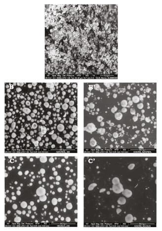
**Figure 5.** ESEM images of pure glyburide (**A**), Aeroperl<sup>®</sup>300 (**B**) and Neusilin<sup>®</sup>US2 (**C**) and of the corresponding liquisolid systems (**B**' and **C**').
