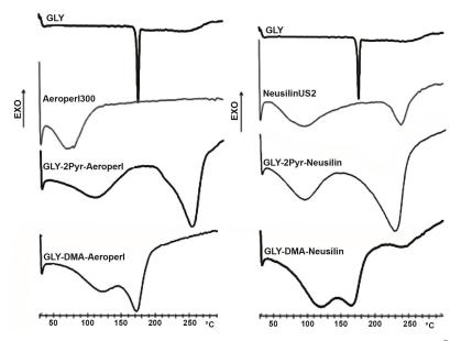
**Figure 3.** Differential Scanning Calorimetry (DSC) curves of pure glyburide (GLY), Aeroperl<sup>®</sup>300 and Neusilin<sup>®</sup>US2 and of the corresponding liquisolid systems with 2-pyrrolidone (2-PYR) or dimetylacetamide (DMA) as non-volatile water miscible solvent.
