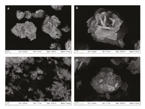
Figure 2. Micrographs obtained by scanning electron microscopy of pristine ZnAl-NO<sub>3</sub> (A,B) and ZnAl-KET (C,D).
