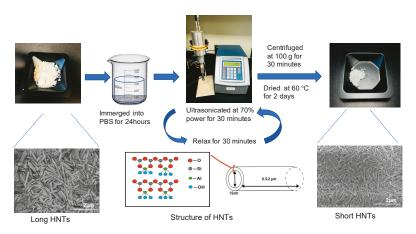
**Figure 1.** The process of reducing the length of halloysite nanotubes (HNTs). Between each step, the composites were washed and filtered using methanol, sodium chloride, a sodium bicarbonate solution, and distilled water (DI).
