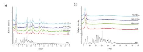
Figure 1. XRPD patterns of the studied samples with sepiolite (a) and montmorillonite (b).
