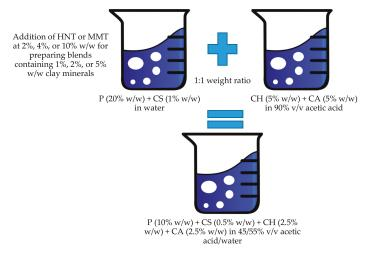
Figure 1. Schematic of the blend preparation.
