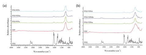
**Figure 4.** Fourier Transform Infrared (FTIR) spectra of sepiolite products (**a**) and of montmorillonite products (**b**).
