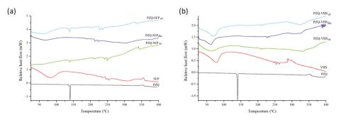
**Figure 2.** Differential Scanning Calorimetric (DSC) profiles of sepiolite and interaction products of sepiolite (**a**) and montmorillonite and interactions products of montmorillonite (**b**).
