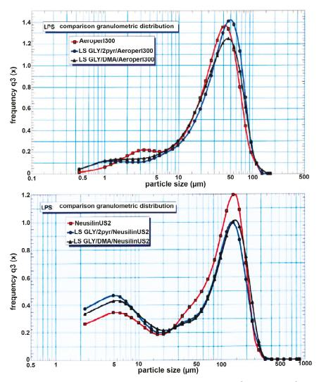
**Figure 2.** Granulometric analysis, by Laser Particle Size (LPS), of pure Aeroperl<sup>®</sup>300 and Neusilin<sup>®</sup>US2, and of the corresponding liquisolid systems with glyburide (GLY) containing 2-pyrrolidone (2-PYR) or dimetylacetamide (DMA) as non-volatile water miscible solvent.
