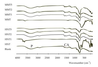
**Figure 4.** Comparison of the FTIR spectra of all the scaffolds developed against to the pristine HNT and MMT. In the blank spectrum the signals related to P (pullulan) and CA (citric acid) are marked.
