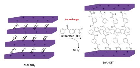
Scheme 1. Schematic representation of the ion exchange between  $NO_3^-$  ions in the pristine ZnAl-HTlc (ZnAl-hydrotalcite) and KET<sup>-</sup> (ketoprofen).
