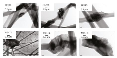
Figure 6. HRTEM microphotographs of the broadened parts of the fibers.
