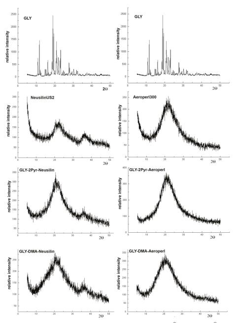
Figure 4. X-Ray powder diffraction patterns of pure glyburide (GLY), Neusilin<sup>®</sup>US2 and Aeroperl<sup>®</sup>300 and of the corresponding liquisolid systems with 2-pyrrolidone (2-PYR) or dimetylacetamide (DMA) as non-volatile water miscible solvent.
