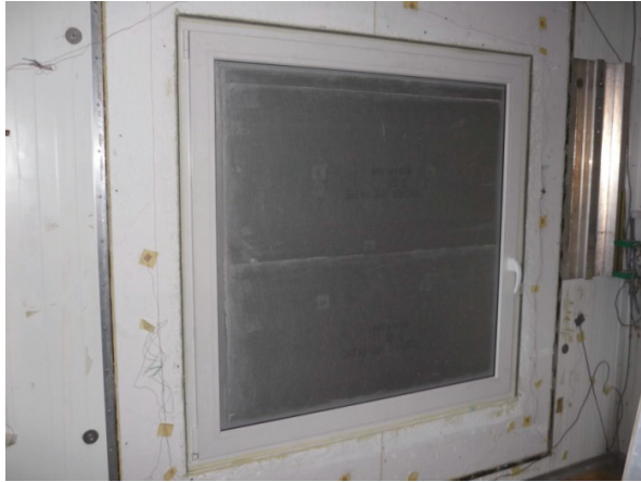
Figure 8. View of the tested window frame in the surround panel on the warm side.
