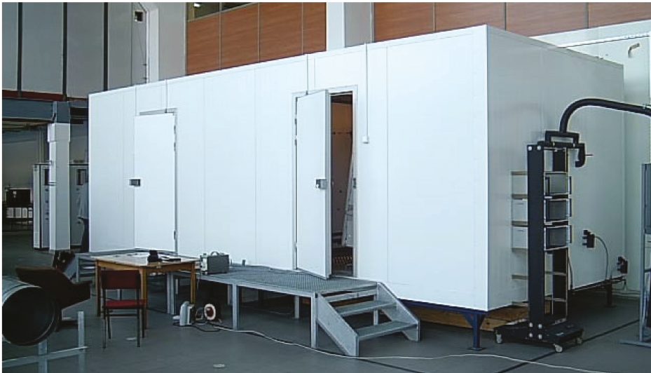
Figure 3. Full-scale climate chambers (cold chamber on the left and warm chamber on the right).
