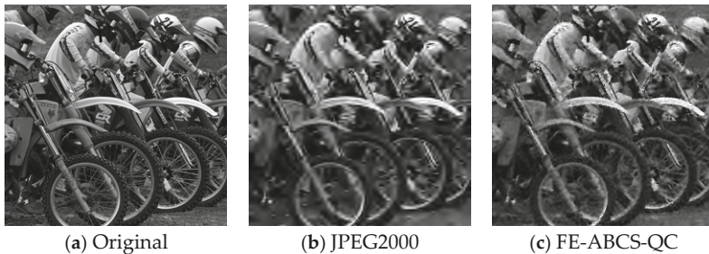
Figure 13. The two algorithms’ comparison of test image Bikes at the condition of \text{bpp} = 0.25 : (a) original image, (b) JPEG2000 image (PSNR = 29.80, SSIM = 0.9069, GMSD = 0.1964), (c) image by the FE-ABCS-QC algorithm (PSNR = 30.50, SSIM = 0.9366, GMSD = 0.1574).
