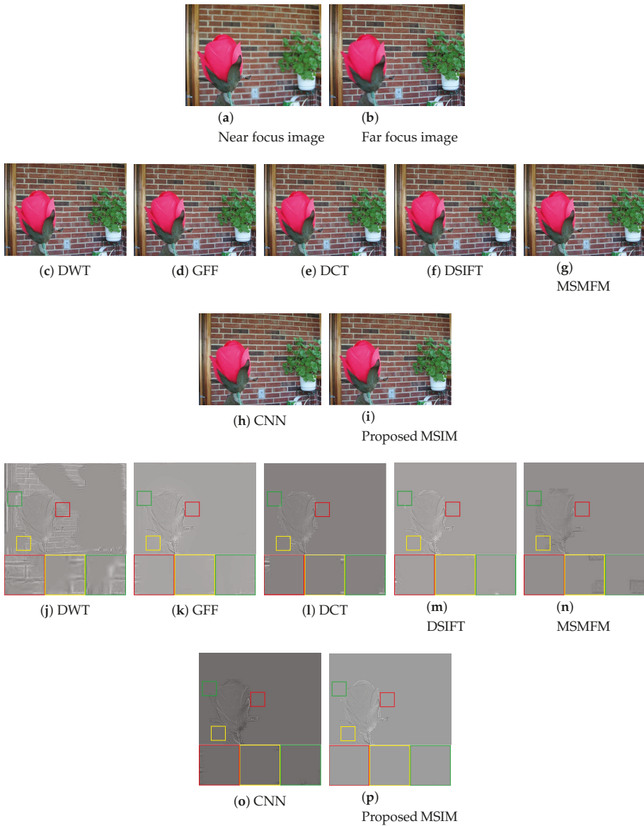
Figure 6. Results of image fusion and their difference images on the “Flower” source images. (c–i) Fused images obtained through fusion schemes. (j–p) Difference images obtained from the fusion results and Figure 6b.
