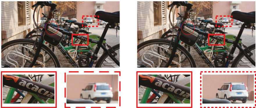
Figure 6. The influence of the aperture size on the image quality. The aperture of the left and right images is set as 4 (large aperture size) and 25 (small aperture size), respectively. The center of the red circle is the location of the focal point. The area surrounded by the solid red box and dotted red box is in foreground and background, respectively.
