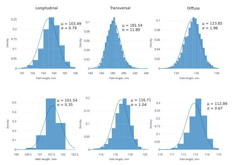
**Figure 10.** Normalized histograms of the shortest path for the longitudinal propagation and transversal propagation for n = 4 node length fibrosis and for n = 1 diffuse fibrosis of the same 30% density in the monolayer (**upper**) and multilayer (**lower**) models. 5000 shortest possible trajectories calculated in 5000 fibrosis matrices are used for each histogram.
