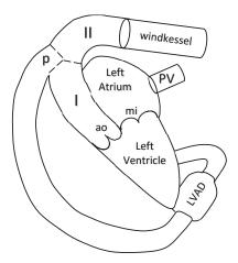
**Figure 1.** Scheme of the integrated model and notations used throughout the paper: left ventricle (lv), left atrium (la), pulmonary veins (pv), mitral valve (mi), aortic valve (ao), Windkessel compartment (WK), left ventricle assist device (LVAD), pump compartment (p).
