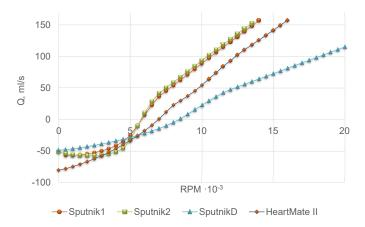
Figure 4. The minimum flow through the pump.
