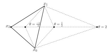
**Figure A2.** Illustration of the Nelder–Mead method. The points  $x_0, x_1$  and  $x_2$  form the initial simplex. The vertex  $x_2$  is replaced with a vertex of the form  $x_{\text{new}} = \bar{x} + \theta(\bar{x} - x_2)$ . If  $f(\hat{x}) < f(x_0)$ ,  $\theta = 2$ , if  $f(x_0) \le f(\hat{x}) < f(x_{n-1})$ ,  $\theta = 1/2$ , and if  $f(x_{n-1}) \le f(\hat{x})$ ,  $\theta = -1/2$ .
