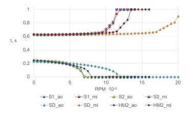
**Figure 3.** Duration of the opening of the aortic and mitral valves. S1—Sputnik 1, S2—Sputnik 2, SD — Sputnik D, HM2 — HeartMate II. The lower index ao stands for aortic valve, mi stands for mitral valve.
