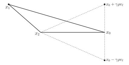
**Figure A5.** Illustration of the new vector  $x^{\Delta}$ , generated to improve the shape of the simplex. The vertex  $x_1$  is replaced with either  $x^{\Delta} = x_0 + \gamma \rho v_{\ell}$  or  $x^{\Delta} = x_0 - \gamma \rho v_{\ell}$ , whichever point results in a smaller value of  $\hat{\Phi}$ .
