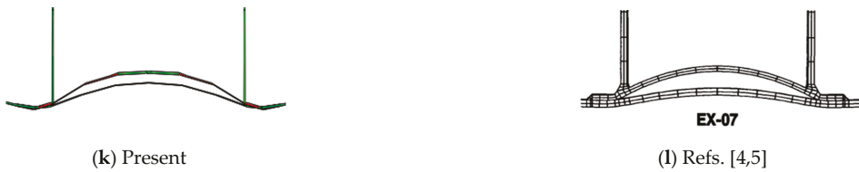
Figure 13. Sliced rings of specimens subjected to compression with \beta = 0.54 : (a) Ex-01 RC, (b) Ex-01 EC, (c) Ex-01 NC, (d) Ex-03 RC, (e) Ex-03 EC, (f) Ex-03 NC, (g) Ex-05 RC, (h) Ex-05 EC, (i) Ex-07 RC, (j) Ex-07EC, (k) particular Ex-07 RC, and (l) particular Ex-07 EC. (With permission from ASCE)
