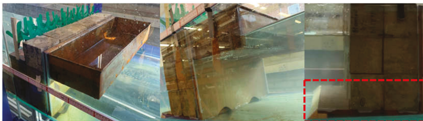
Figure 4. Overtopping collection device. The red box highlights the testing platform.
