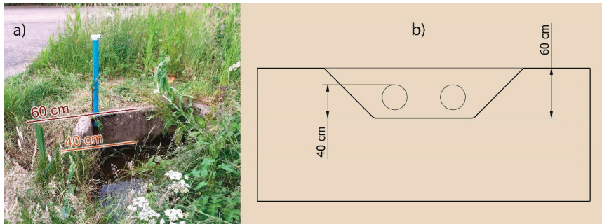
Figure 3. Water levels of hydraulic failure indicated at the discharge point (a) and its cross section (b).
