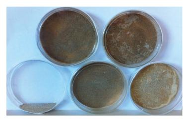
**Figure 6.** Samples of biocemented sand through CaCO<sub>3</sub> precipitation by strains P2, P11, M5, and P9 (starting from the **upper left** to the **lower right**) after 20 days of incubation, at 28 °C. Untreated control at the **left bottom**. The plates were positioned vertically to highlight the biocementation of the sand, not present in the control.
