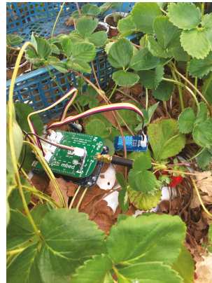
(b) LoRa Node, sensors and strawberry plant.
