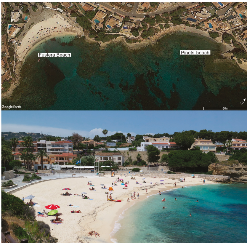
Figure 7. Fustera Beach nourished in 2017 with quarry sand (No. 51, Table A1), and Pinets beach, non-altered site. The contrast between the artificial beach vs the natural one is obvious (2018 year). The bottom of the figure shows Fustera Beach in summer 2017.
