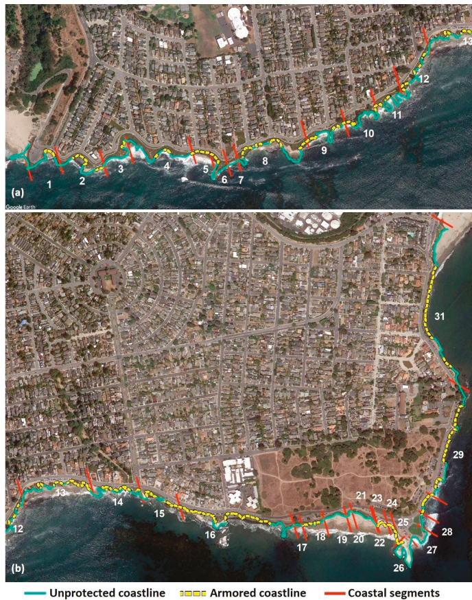
Figure 13. Map of the 31 identified coastal segments, armored coastline, and unprotected areas along the West Cliff Drive coast—(a) West side (b) East side.
