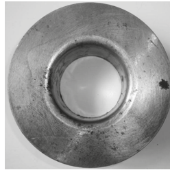
Figure 6. Active die used for manufacturing the test parts.
