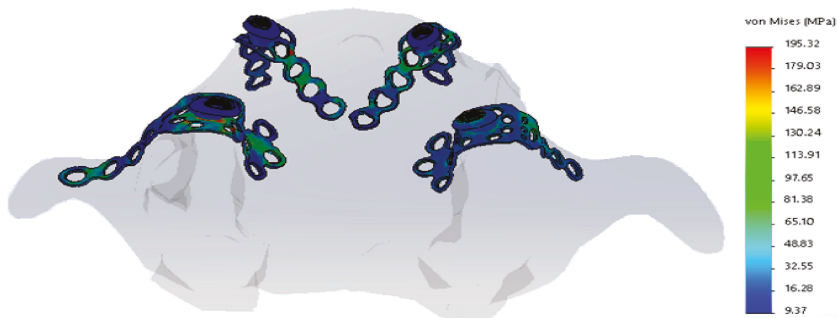
Figure 9. The von Mises stress on plates in MPa.
