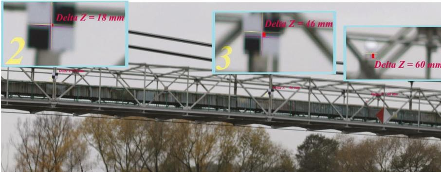
**Figure 12.** Bridge deflections under static loading (A) obtained from the photogrammetry.
