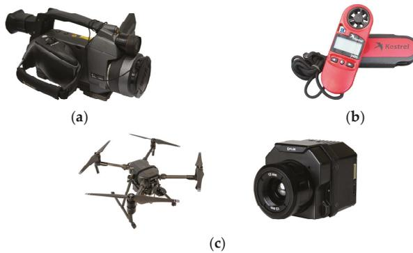
**Figure 9.** Equipment used in the experiment: (a) H-IRC; (b) Kestrel 3000; (c) UAV-IRC.
