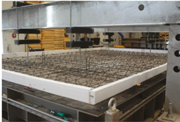
**Figure 2.** Structure and distribution of the reinforcement.
