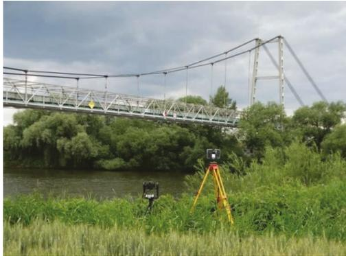
**Figure 8.** Side view of the bridge measurement sets for laser scanning and photogrammetry.
