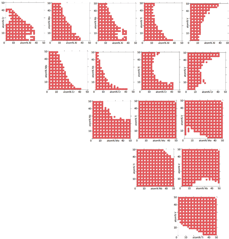
Figure 7. Two-dimensional projections for Al_3Cr_6Mo_6Nb_6Ti_6V_{1-a-b-c-d-e-v} , showing at which concentrations for two elements the alloy forms a bcc HEA at 800 K. Four concentration dimensions are flattened out to arrive at the two-dimensional projection. The concentrations of the four elements not shown are as explained in the caption of Figure 2. The concentration increments are 4%.
