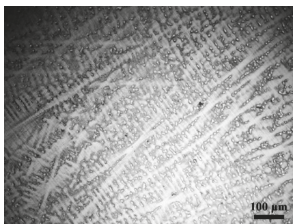
Figure 1. Optical micrograph of the as-cast NiCrFeCoMn alloy.
