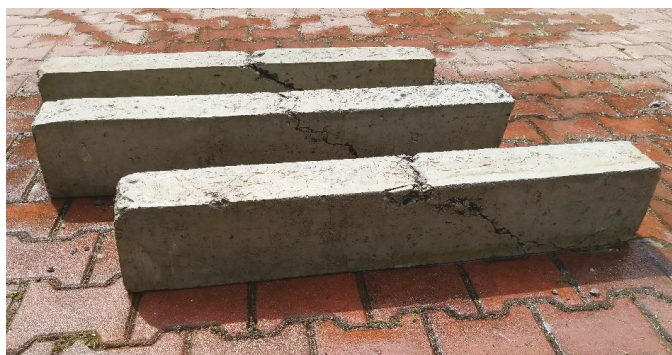
Figure 20. Reinforced concrete (RC) Beams with shear crack.
