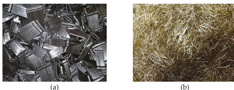
Figure 4. Steel fibers: (a) Dramix® 3D 55/30 BG (hooked fibers); (b) Dramix® OL 13/20 (straight fibers).
