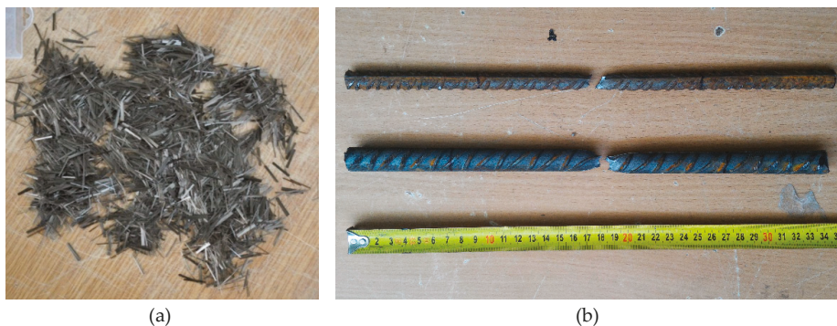
Figure 1. (a) Fibres used in experimental work; (b) reinforcing bars after tensile test.
