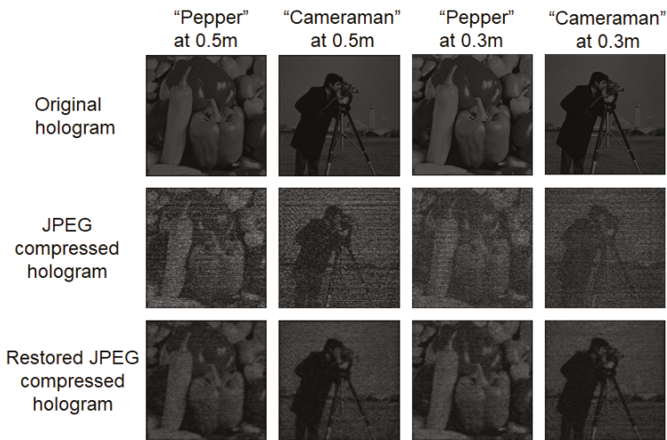
Figure 8. Reconstructed images from original holograms, JPEG compressed holograms and restored holograms in numerical simulation.
