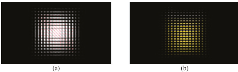
Figure 3. Two captured EIAs from each of the two different 3-D objects of ‘Dice’ and ‘Car’ on the on-axis integral imaging system (a) captured EIA from the ‘Dice’ (b) captured EIA from the ‘Car’.
