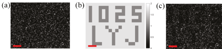
Figure 6. (a) Intensity (amplitude) distribution of the illumination wave. (b) Amplitude of the object. (c) Amplitude of the reflected wave. Scale bar: 550 \mu\text{m} .
