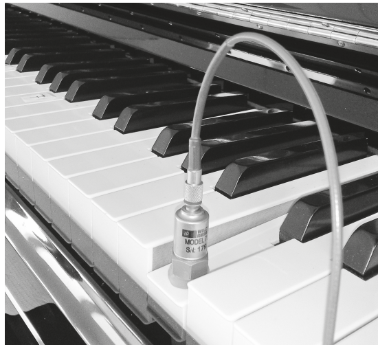
Figure 2. Vibration recording setup. A Wilcoxon Research 736 accelerometer is attached with adhesive tape to a key that is being played remotely via MIDI control.
