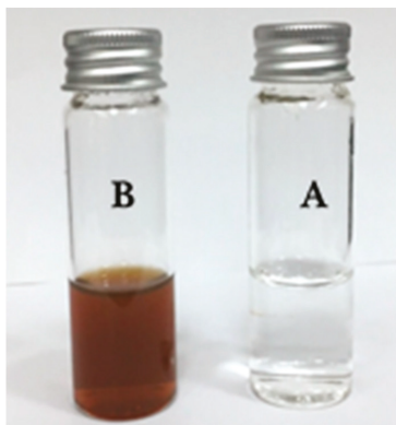
Figure 1. Color and appearance changes during synthesis of silver nanoparticles (Ag NPs) using J. regia leaf extract. J. regia leaf extract containing silver nitrate before (A) and after (B) exposure to microwave irradiation.
