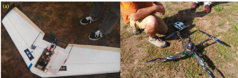
Figure 1. The unmanned aerial vehicles (UAVs) before launch. (a,b) are the fixed-wing and rotor wing UAVs for Brooksvale Park and Yale Playground, respectively.
