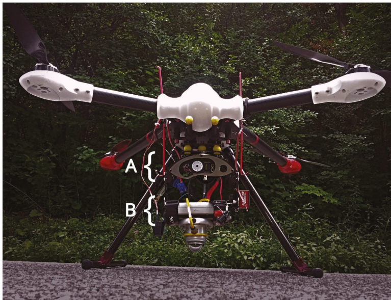
Figure 2. Preparation of the UAV for flight. The gimbal (A) is visible underneath the UAV, equipped with the downward-facing pyranometer secured beneath (B).
