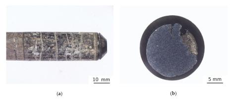
**Figure 5.** The microstructure of the hot swaged (HEAP-S-SW) specimen: (a) overview with radial cracks; (b) after forging in Ti-envelope.
