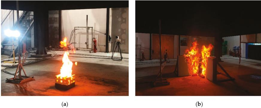
Figure 2. Independent measurement of heat release rate for (a) the wood crib and (b) polyether foam.
