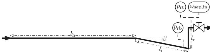
**Figure 3.** Drawing of the well-pipeline-riser test facility.
