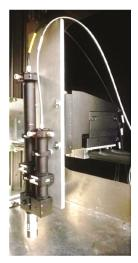
Figure 9. Raman scanning probe with long working distance mounted on a 3D-displaceable table [24].
