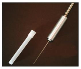
Figure 5. Cannula sterican 19G, 30° bevel [4].
