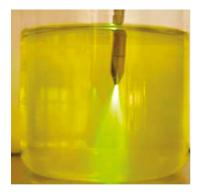
Figure 6. Tyndall effect, 10 ppm fluorescein sodium in water [4].
