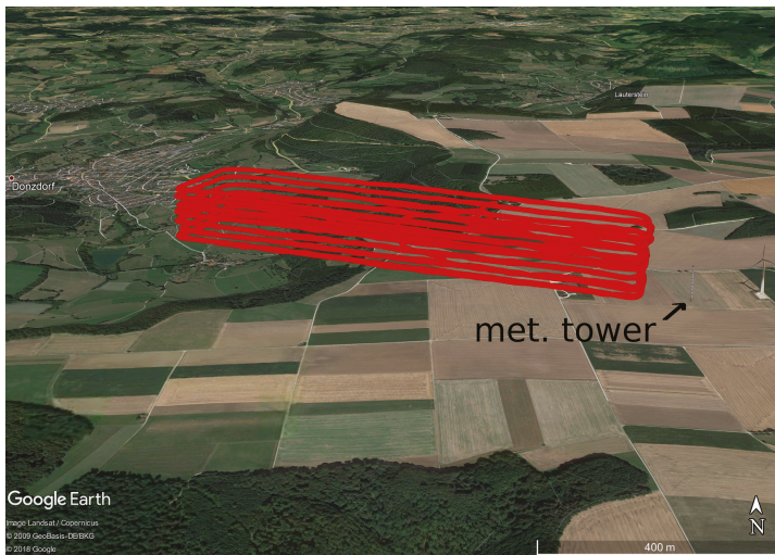
Figure 7. Flight path (so-called racetracks) in red in Schmittlingen (SNT) on 7 May 2015, with the meteorological tower east of the flight path. During the measurement, moderate westerly winds prevailed. The crest forms partial up-drafts and strongly sheared flow.
