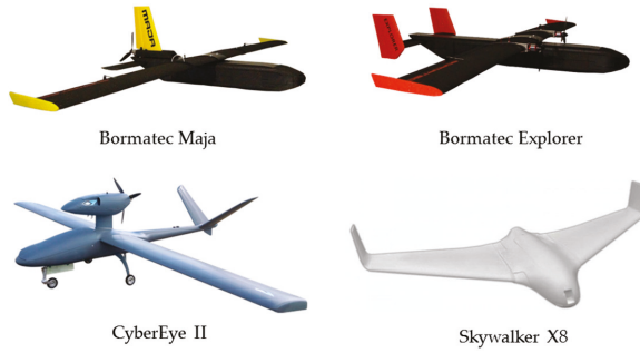
Figure 1. Examples of fixed-wing unmanned aerial systems (UAS) platforms for trace gas monitoring.
