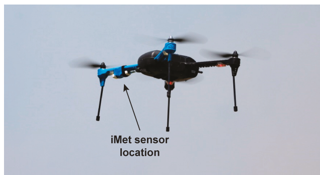
Figure 2. Location of iMet XQ sensor mounted on underside of 3DR Iris+ multirotor platform.
