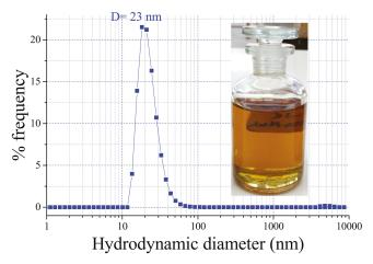
**Figure 1.** Size distribution diagram based on dynamic light scattering measurement of the colloidal magnetic iron oxides nanoparticles (MIONs) in the oil matrix and digital image colloidal nanofluid (colNF) after 2 months of storage (inset).
