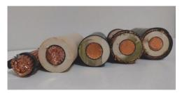
Figure 2. Cable layers.
