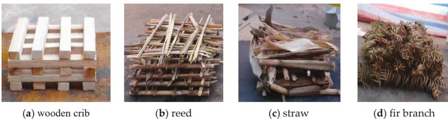
Figure 2. Arrangement of typical vegetation.
