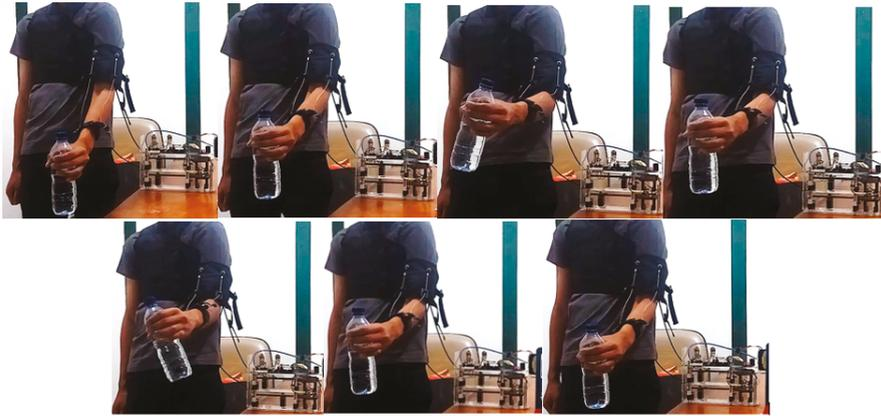
**Figure 17.** Sequence images of two DOF mechanical assistance for flexion/extension and pronation/supination motion.
