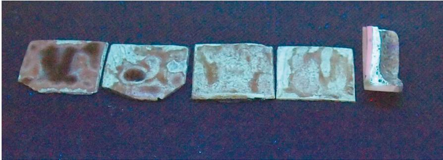
**Figure 8.** From the left: Coatings after CMAS interaction for 1, 4, 8 and 10 h and the cross-sectioned bottom of a crucible with sintered mixture of powders, respectively. Samples illuminated by the 312 nm lamp (i.e., 3.97 eV).
