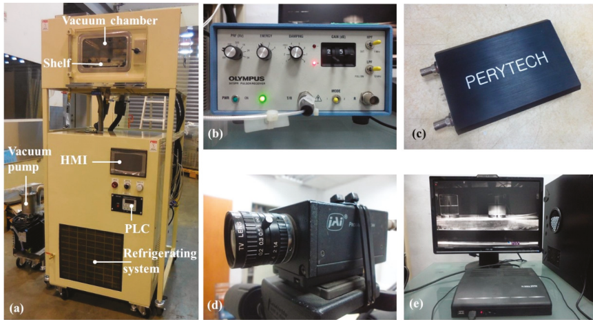
Figure 4. Photographs of (a) the split-type freeze-drying machine with vacuum chamber, controller unit, refrigeration unit and vacuum pump, (b) the ultrasonic pulse/receive unit, (c) a PC-based digital oscilloscope, (d) Charge-coupled device (CCD) camera, (e) digital video recorder (DVR) and PC.
