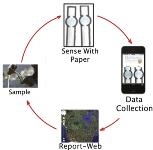
Figure 15. Concept of water quality evaluation using paper-based colorimetric sensors and a smartphone. Reprinted from Water Research, Vol. 70, Clemence Sicard, Chad Glen, Brandon Aubie, Dan Wallace, Sana Jahanshahi-Anbuh, Kevin Pennings, Glen T. Daigger, Robert Pelton, John D. Brennan, Carlos D.M. Filipe, Tools for water quality monitoring and mapping using paper-based sensors and cell phones, Pages 360–369, Copyright (2015), with permission from Elsevier.
