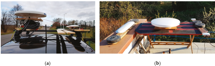
Figure 6. Experimental setup: (a) on a car roof for the automotive tests; (b) on a house roof for the stationary sets. Photo: K. Zwolak.
