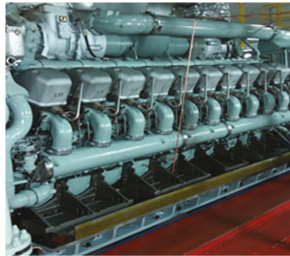
Figure 12. The diesel engine with 20 cylinders.
