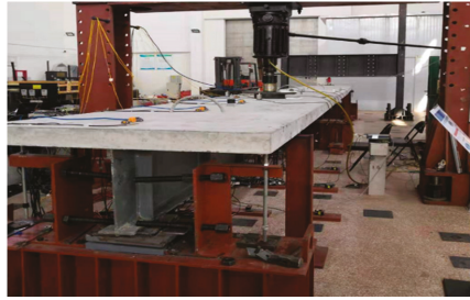
Figure 3. Verified by fatigue tests on bridge model.
