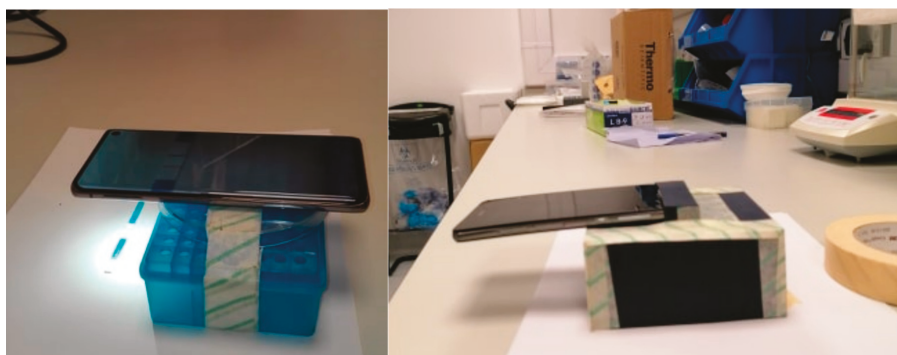
Figure 4. Left; an image of the Samsung taking an image of a LFA (the ZEU Proteon Gluten Express) under room-light conditions with the flashlight on at 5 cm distance. Right; an image of the light-shielding box used. The dimensions of the box are 11 \times 11 \times 5 cm to maintain the standard 5 cm as a distance for the photo capturing. The box had a hole in the center precisely for the camera and flash. The phone displayed on the box is the Huawei.
