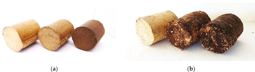
Figure 6. Visual comparison of produced bio-briquette samples: (a) A + B mixtures; (b) A + C mixtures.
