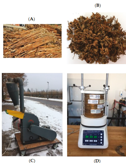
Figure 1. (A) Sunflower stalks and (B) hazelnut husks. (C) A 5.5 kW motor hammer mill (9FQ-40C, Pest Control Corporation, s.r.o., Vlčnov, Czech Republic) used to grind the biomass materials. (D) A sieve shaker (AS 200, Retsch, Haan, Germany) of four sieve opening sizes.
