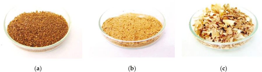
Figure 1. Feedstock samples: (a) spent coffee ground (sample A); (b) larch sawdust (sample B); (c) spruce shavings (sample C).
