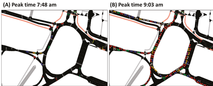
Figure 7. Comparison of Traffic Volumes at peak times for (A) 5000 journeys and (B) 10,000 journey scenarios.
