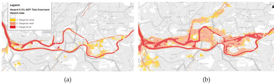
Figure 7. Hazard mapping for the 0.5% AEP tidal/fluviat event in (a) Present day (left) (b) 2115 (inclusive of climate change) (right).
