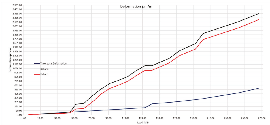
Figure 23. Theoretical deformation of the rebars compared with the real deformation obtained using the optic fiber sensors.
