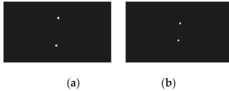
Figure 3. Laser points with different distances between the camera plane and the target plane: (a) 200 mm and (b) 350 mm.
