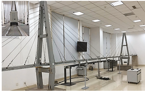
Figure 1. Experimental platform for testing continuous deflection.
