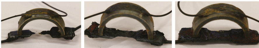
Figure 14. The three corrosion sensors after accelerated corrosion failure.
