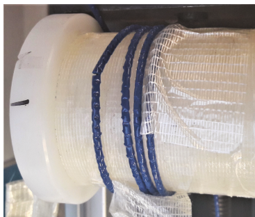
Figure 5. Impact of the radiation on the cable: radiation reduces the elasticity of the plastic, causing cracks when curved.
