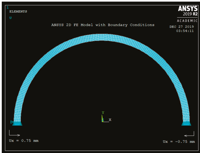
Figure 6. ANSYS Finite Element (FE) Model.
