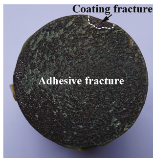
Figure 5. Fracture of tensile test specimen.
