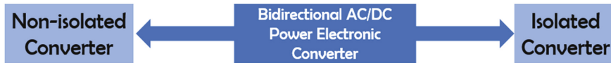
Figure 9. Classification of bidirectional AC/DC power converter topologies: the bidirectional AC/DC power electronic converters are mainly of two types, isolated and non-isolated converters.
