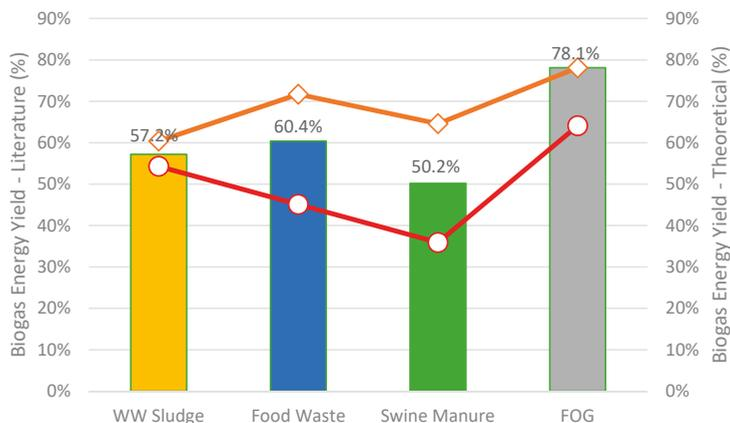
**Figure 6.** Biogas Energy Yield (%) from Wet Waste Feedstocks. The bar chart shows the theoretical values of energy yield from different wastes while the line chart shows the range of energy yields from the literature.
