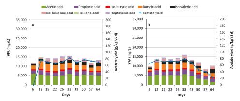
Figure 2. Volatile fatty acid (VFA) composition and acetate yield in reactors (a) CO-S (reactor inoculated from co-digestion plant fed with sewage sludge) and (b) WW-S (reactor inoculated from wastewater treatment plant fed with sewage sludge).
