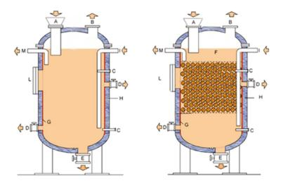
**Figure 1.** Schematic of the digesters D1 (left) and D2 (right): solid materials input (blocked in the present experimentation) (A), biogas output (B), temperature probe housings (C), sampling points (D), bottom discharge (blocked) (E), fixed bed (F), heating coil (G), insulation (H), sludge input and recirculation ports (I), maintenance openings (L) and digestate output (M).
