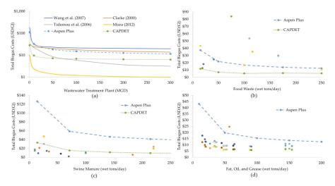
**Figure 7.** Total Biogas Production Costs in USD/GJ for AD Processing (a) Wastewater Treatment Sludge, (b) Food Waste, (c) Swine Manure, and (d) Fat, Oil, and Grease. Please note that that *y*-axis on Figure 7a is plotted on a log-scale.
