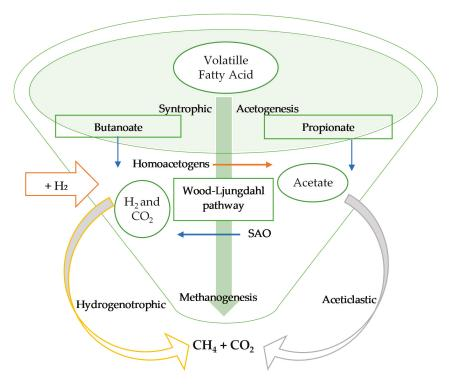
Figure 7. Metabolic pathways for hydrogen assisted methanogenesis [25].
