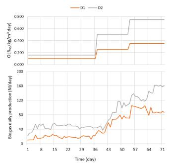
Figure 3. Evolution of OLR<sub>VS</sub> (above) and of daily biogas production (below).
