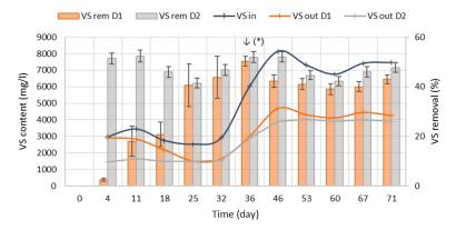
**Figure 2.** Evolution of VS concentration in the input and in digestates from D1 and D2, and of VS removal rates.  $\downarrow$ (\*) = implementation of influent sedimentation.
