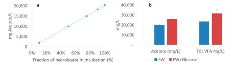
Figure 4. (a) Correlation between fraction of hydrolysate after two days of inoculation and absolute acetate concentration ( $R^2 = 0.9997$ ). (b) Concentration of acetate and total volatile fatty acids (VFA) with only food waste (FW) (blue) compared with FW plus extra dissolved organic carbon (red).
