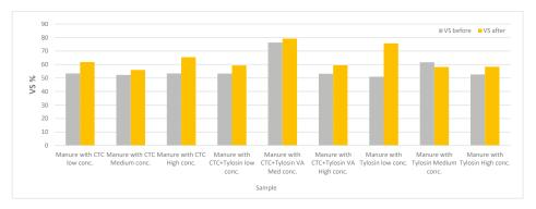
Figure 5. Digestate volatile solid (VS) concentrations before and after VA additions.
