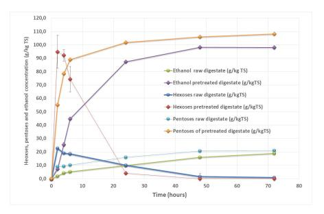
**Figure 3.** Hexose consumption and ethanol production for raw solid separated digestate and pretreated solid separated digestate with VBM for 30 min.
