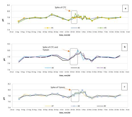
**Figure 3.** Digestate pH levels for (a) before and after CTC spike, (b) before and after CTC plus tylosin spike, and (c) before and after tylosin spike and the dotted box shows the administration period of the VAs.
