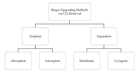
Figure 1. Technologies for biogas upgrading via CO<sub>2</sub> removal route.
