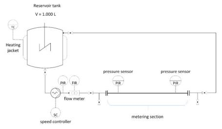
Figure 2. Scheme of the pipe viscometer.
