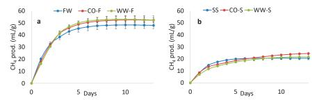
**Figure 8.** Volumetric bio-methane production from (a) food waste (FW) and hydrolysate from reactors CO-F and WW-F, and (b) sewage sludge (SS) and hydrolysate from reactors CO-S and WW-S. Error bars indicate the calculated standard deviation for daily values.
