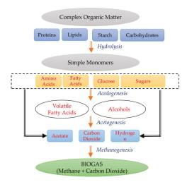
Figure 2. Steps in the Anaerobic Digestion Process.
