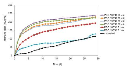
Figure 1. Methane yields in BMP tests.
