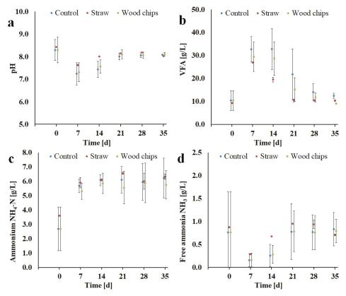
**Figure 4. a–d.** Process conditions during dry batch anaerobic digestion of chicken manure. pH value (a), volatile fatty acid concentration (b), ammonium concentration (c), free ammonia concentration (d).
