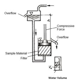
Figure 1. Schematic illustration of the oedometer testing appartus.
