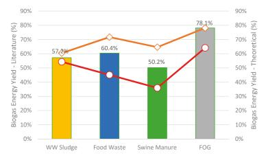
**Figure 6.** Biogas Energy Yield (%) from Wet Waste Feedstocks. The bar chart shows the theoretical values of energy yield from different wastes while the line chart shows the range of energy yields from the literature.
