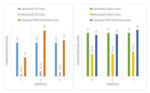
**Figure 7. Left:** concentrations of CTC, comparing calculated, measured, and corrected concentrations. **Right:** concentrations of tylosin, comparing calculated, measured, and corrected concentrations.
