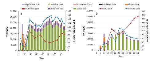
**Figure 1.** Volatile fatty acid (VFA) composition and acetate yield in reactors (a) CO-F (reactor inoculated from co-digestion plant fed with food waste) and (b) WW-F (reactor inoculated from wastewater treatment plant fed with food waste).
