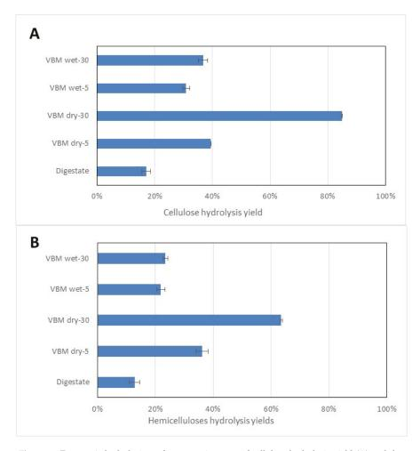
**Figure 2.** Enzymatic hydrolysis performances in terms of cellulose hydrolysis yield **(A)** and the hemicelluloses hydrolysis yields **(B)** for raw SS-DIG and vibro-ball milling (VBM)-pretreated samples in wet and dry modes.
