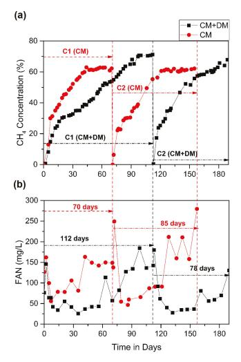
**Figure 7.** Comparative study of chicken manure (CM) mono-digestion and CM + dairy cow manure (DM) co-digestion: (a) Methane concentration profile; (b) FAN profile.
