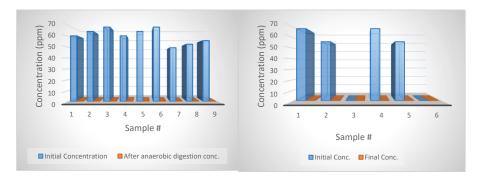
Figure 8. Left: CTC concentration change with anaerobic digestion. Right: CTC concentration change with reactors filled with diluted water.
