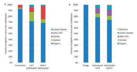
**Figure 3.** Composition of ingoing substrate and outgoing hydrolysate from reactors fed (a) food waste (CO-F, WW-F) and (b) sewage sludge (CO-S, WW-S). Mass of outgoing gases is included in the hydrolysate.
