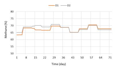
Figure 4. Evolution of methane concentration in biogas.
