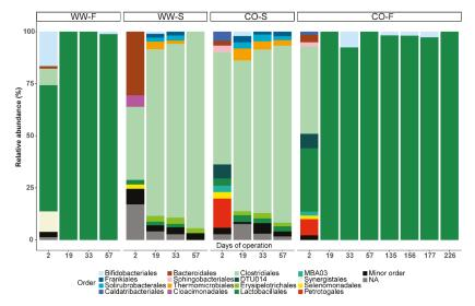
**Figure 7.** Relative abundance of microbial order (based on total bacterial and archaeal sequences) in reactors inoculated with sludge from the co-digestion plant (CO) or an anaerobic digestion process fed mixed sludge (WW) and fed food waste (F) or sewage sludge (S). Days of operation at the point of sampling are given on the *x*-axis.
