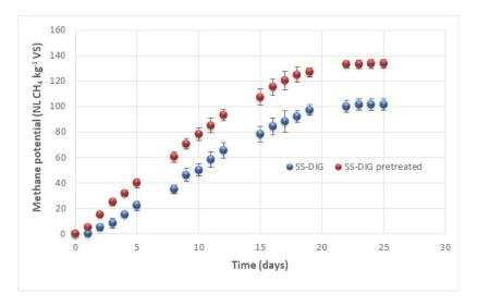
**Figure 4.** Methane potential (NL  $CH_4$  kg<sup>-1</sup> VS) of raw SS-DIG and pretreated SS-DIG by VBM at 30 min.
