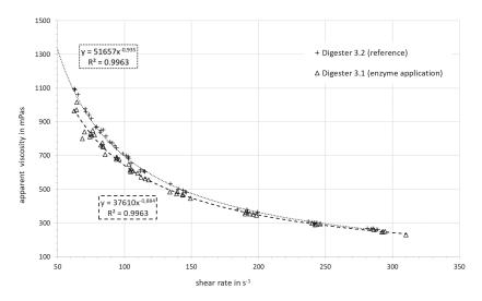
**Figure 7.** Apparent viscosity vs. the shear rate: comparison of digester slurry with and without enzyme addition.
