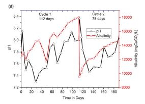
**Figure 2.** Performance of the liquid and solid digesters at different organic loading rates (OLRs) during 190 days of operation. (a) Biogas production rate; (b) Biogas composition; (c) Specific methane yield (SMY); (d) pH and alkalinity profiles.
