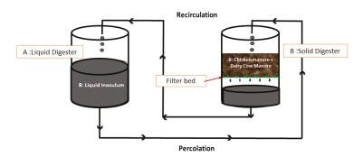
Figure 1. Schematic diagram of a single set of two-stage (liquid-solid) digesters.
