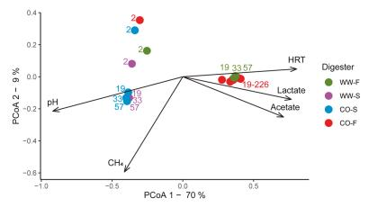
**Figure 5.** Principal coordinate analysis (PCoA) plot of microbial community structure using weighted UniFrac. Reactor parameters significantly associated with changes in microbial community structure are plotted as vectors, where the length and direction indicate the contribution of the variable to the principal components. Variable HRT stands for hydraulic retention time.
