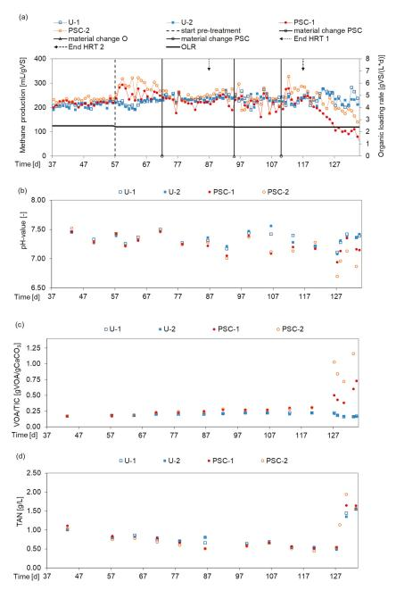
**Figure 3.** (a) Methane production of cattle manure in semi-continuously stirred tank reactor (CSTR) (U = untreated, PSC = pressure swing conditioning); (b) pH-value; (c) volatile organic acids and total inorganic carbon (VOA/TIC); (d) total ammonia nitrogen (TAN).
