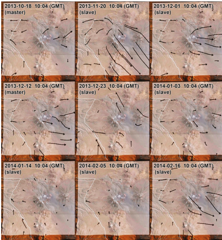
Figure A2. Time series of surface wind fields obtained from the lowest eta level of WRF, determined for acquisition times of each SAR image. Katabatic (downslope) mountain winds prevail at the time of SAR acquisitions, which were recorded during the early morning hours at about 10:04 a.m. (UTC), respectively 07:04 a.m. (CLST).
