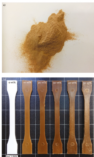
Figure 1. (a) Powdered almond shell flour (ASF) and (b) injection moulded PBS/ASF/MLO composites with varying ASF content in wt%.
