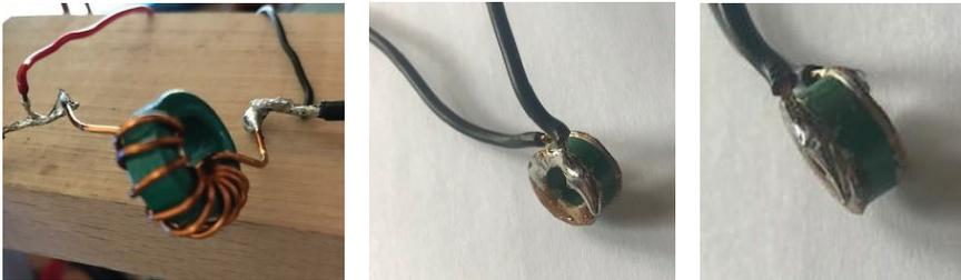
Figure 5. Tested inductors containing toroidal cores.
